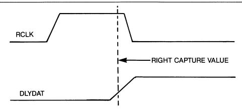
Continue moving DLYDAT to the left until the WD1001 fails again. Move DLYDAT to the right until the controller functions again. This is the left capture value.
